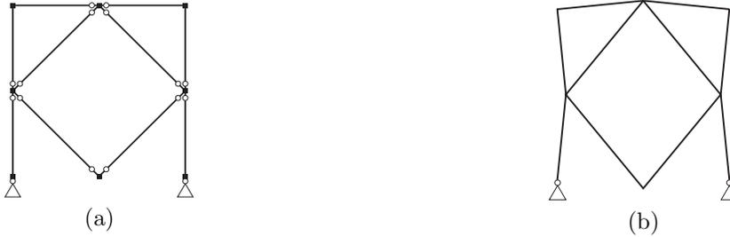
Figure 6: Symmetric finite mechanism of the  $2 \times 2$  grid; removed members are not shown: (a) locations of hinges, (b) inextensional deformation.
