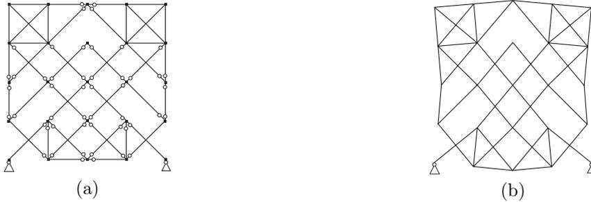
Figure 10: Symmetric finite mechanism of the  $4 \times 4$  grid; removed members are not shown: (a) locations of hinges, (b) inextensional deformation.
