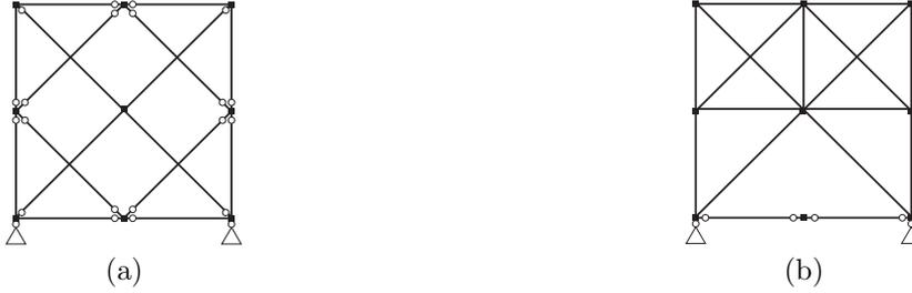
Figure 4: Locations of hinges of infinitesimal mechanisms of the planar  $2 \times 2$  grid; removed members are not shown: (a)  $0.414 \leq \alpha \leq 0.630$ , (b)  $\alpha \geq 0.631$ .
