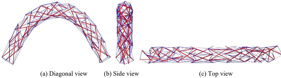
Figure 4. Self-equilibrated tensegrity arch by dynamic relaxation method.
