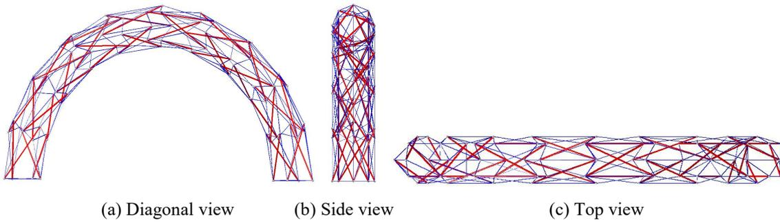
Figure 3. Initial configuration of the tensegrity arch.
