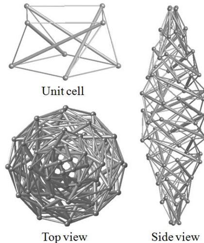
Figure 1: Self-equilibrium configuration of the ten-layer tensegrity tower by force density method.
