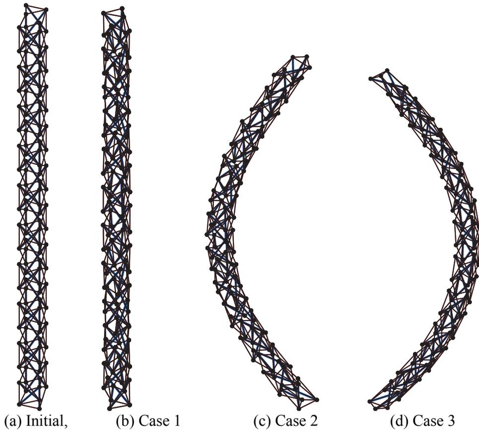
**Figure 2. Initial and self-equilibrium shapes of a 20-layer tensegrity tower.**
