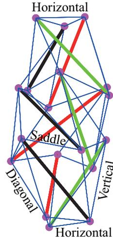
**Figure 1. A 3-layer tensegrity tower model.**
