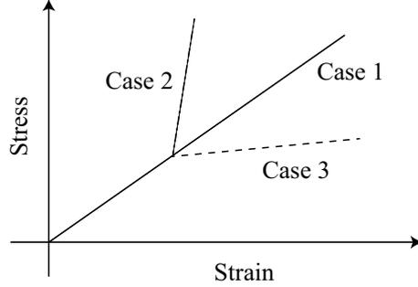
**Figure 3. Bilinear stress-strain relations.**
