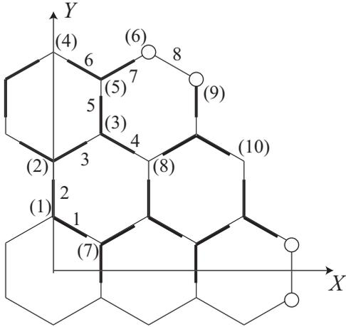
Fig. 5: Node numbers (with parentheses) and member numbers (without parentheses) of one of 12 equal parts of the 3-layer hexagonal latticed shell
