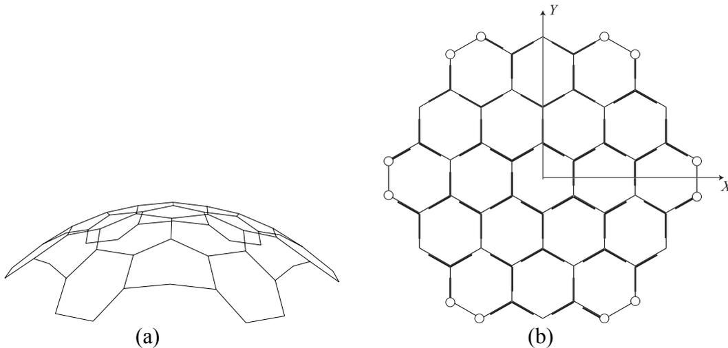
Fig.1: A hexagonal-grid latticed shell ( $D=3$ ); (a) diagonal view, (b) assemblage of units
