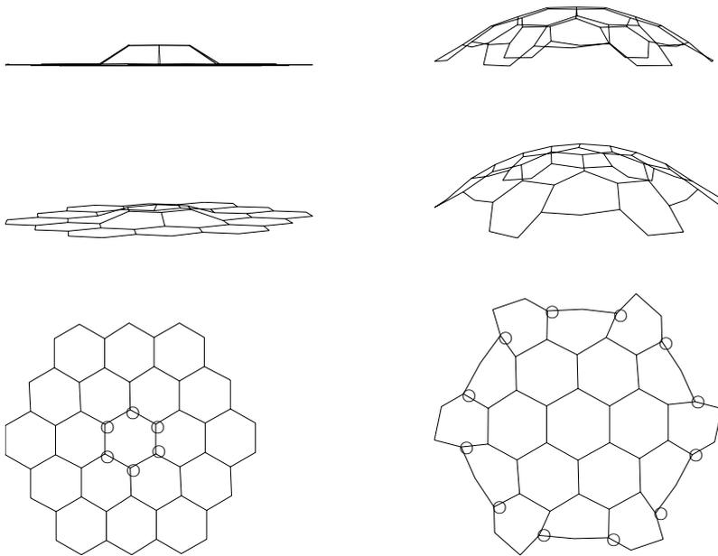
Fig 7: Configuration during lift-up process; (a) after 1st step, (b) after 4th step
