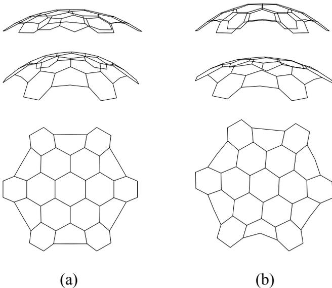
Fig. 6: Deformation for Case 2 under uniform vertical loads; (a) undeformed, (b) deformed
