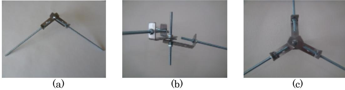
Fig. 8: Connections of members; (a) a unit consisting of two bars, (b) center of unit, (c) connection between units
