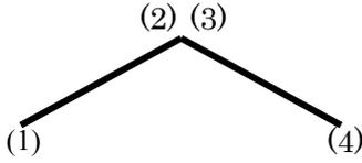
Fig. 3: A unit consisting of a pair of members, and its member-end numbers
