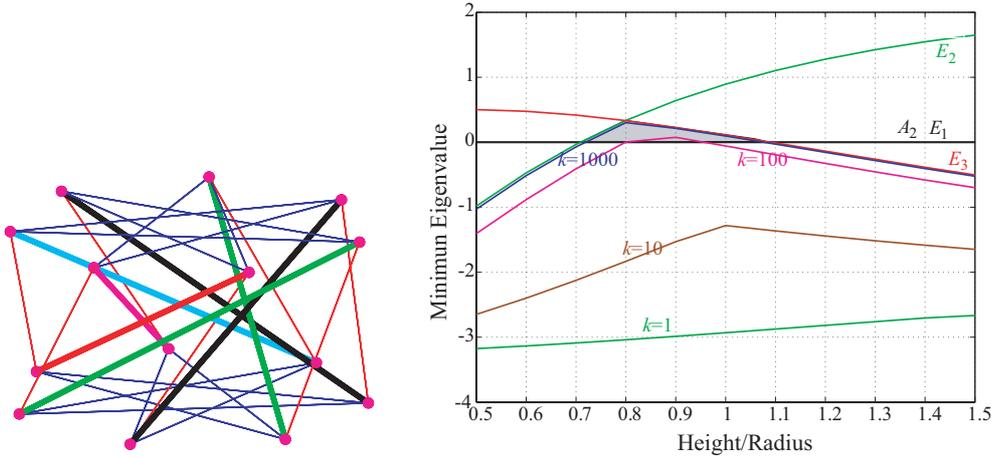
Fig. 6: The influence of the height/radius ratio and the stiffness/prestress ratio  $k$  on the stability of the structure  $\mathbf{D}_7^{3,2}$ .
