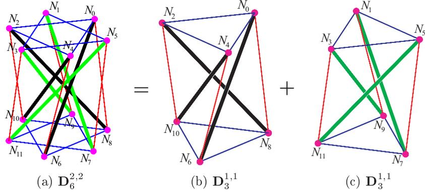
Fig. 3: An example of divisible structure  $\mathbf{D}_6^{2,2}$  and its two substructures  $\mathbf{D}_3^{1,1}$ .
